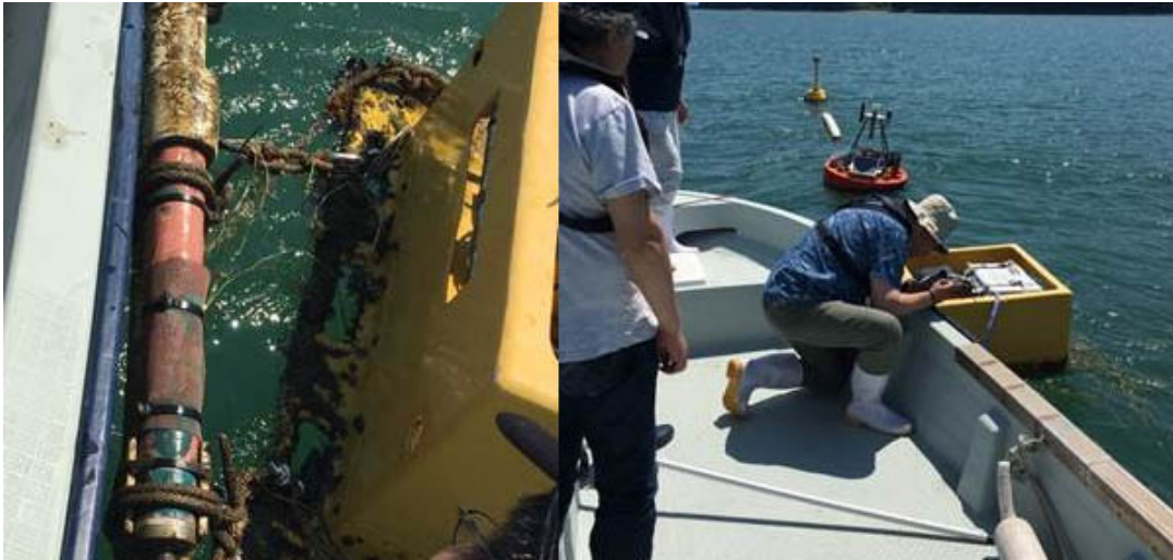
Above left: Inspecting SUNA V2 after 3 week deployment. Above right: Checking buoy line with SUNA V2 nitrate analyzer.
